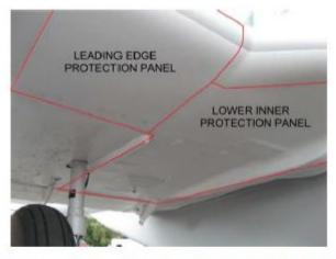
FIGURE 4 LOWER WING SURFACE (SHORT RANGE WING)
