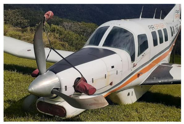
Figure 4: Propeller damage.
