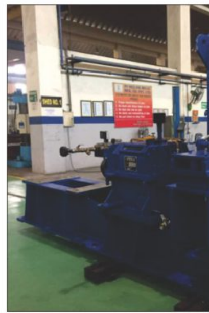
Combination Shear with 8mm @ 40mps
