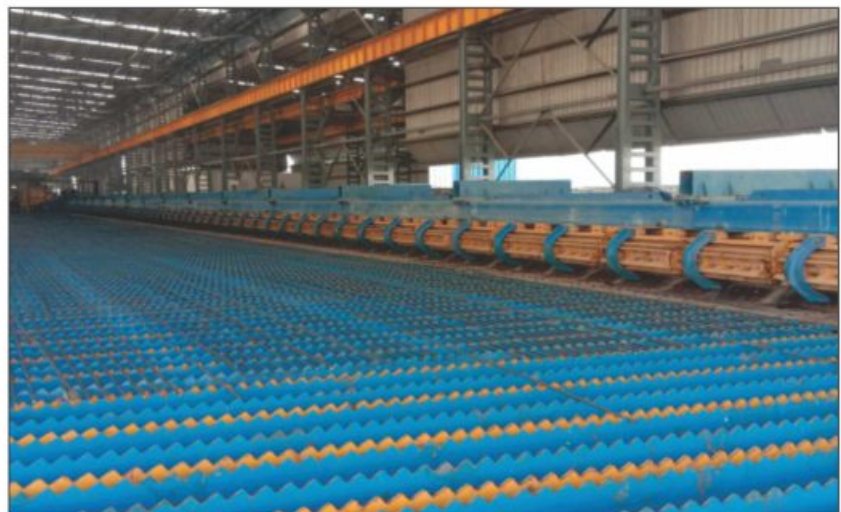
High Speed Rotating Drums can handle 8mm Rebars at 40 mps
