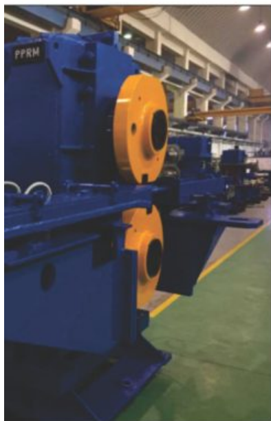
to cut 8 mm to 40mm and 40mm @ 2mps
