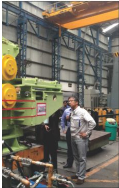
Shear to cut 8mm in High Speed KOBELCO Japan
